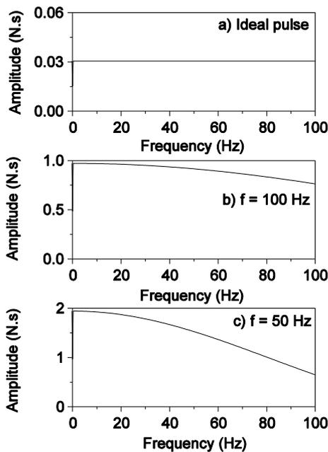
Fig. 4 Fourier spectrum of the time histories of the imaginary impact forces: a) ideal impact force, b) impact force with smaller contact duration, and c) impact force with longer contact duration.
