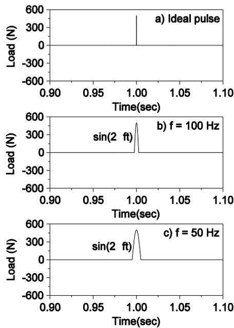
Fig. 3 Time histories of the imaginary impact forces: a) ideal impact force, b) impact force with smaller contact duration, and c) impact force with longer contact duration.
