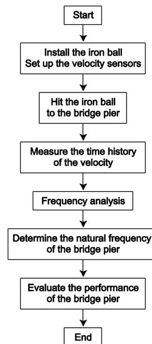
Fig. 1 Flow chart of the conventional percussion test.
