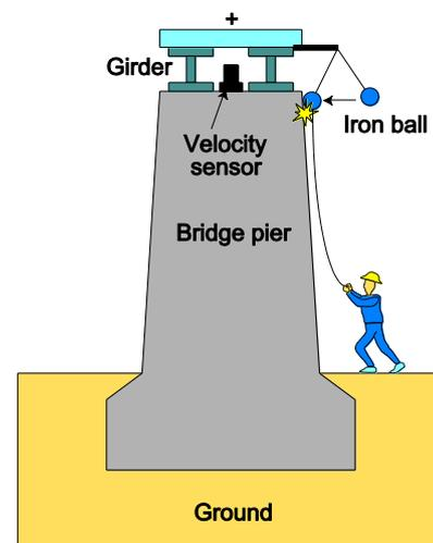
Fig. 2 Typical percussion test.
