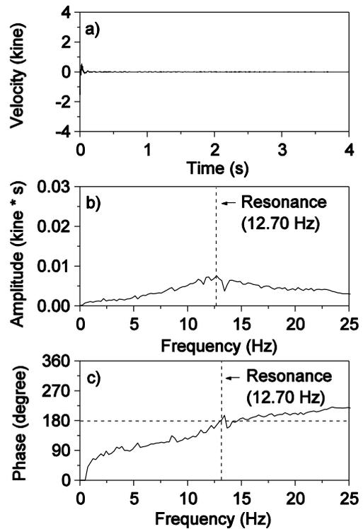
Figure 11 Result of the impact vibration test of the pier C and its foundation: a) time history of the velocity at the top of the pier C, b) Fourier spectrum of the time history of the velocity and c) phase spectrum of the time history of the velocity.
