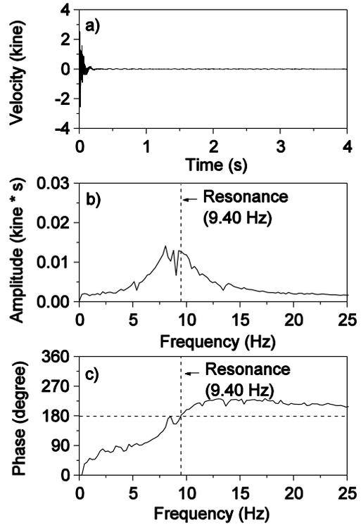
Figure 10 Result of the impact vibration test of the pier B and its foundation: a) time history of the velocity at the top of the pier B, b) Fourier spectrum of the time history of the velocity and c) phase spectrum of the time history of the velocity.
