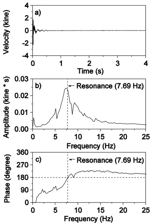
Figure 9 Result of the impact vibration test of the pier A and its foundation: a) time history of the velocity at the top of the pier A, b) Fourier spectrum of the time history of the velocity and c) phase spectrum of the time history of the velocity.
