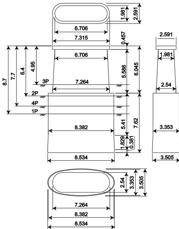
Fig. 7 Schematic figure of the pier and caisson.
