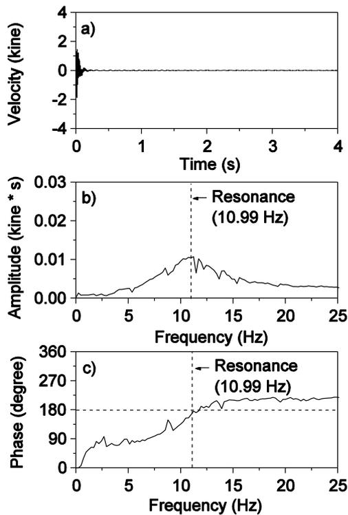
Figure 12 Result of the impact vibration test of the pier D and its foundation: a) time history of the velocity at the top of the pier D, b) Fourier spectrum of the time history of the velocity and c) phase spectrum of the time history of the velocity.
