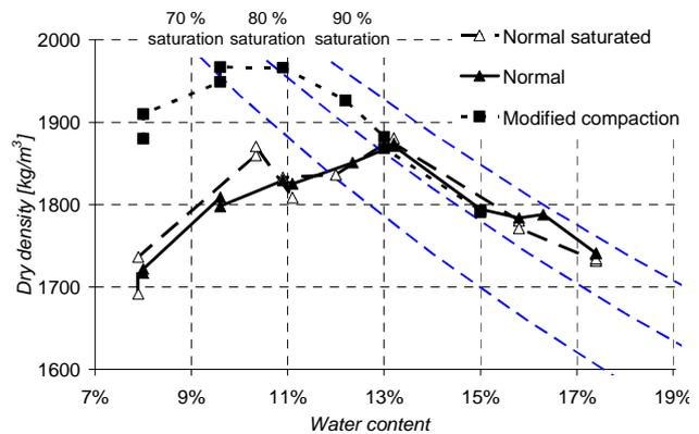
Figure 2 Dry density versus water content at compaction for the P2 soil.
