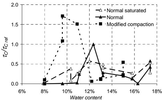
**Figure 5** Relative variation of the critical shear stress  $\tau_c$  for the P2 soil according to the water content at compaction.
