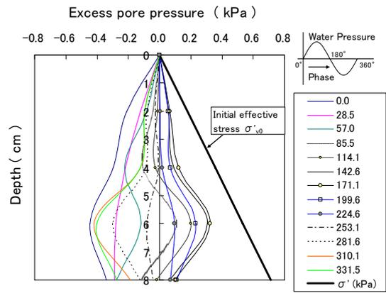
Fig. 6 (b) Excess Pore pressure during 1-D cyclic water pressure changes (Clay2-SF8, unsaturated, after 12 hour)
