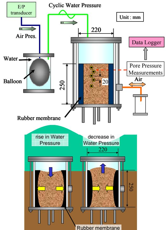
Fig. 8 Test Apparatus for Cyclic Water Pressure Changes with Lateral displacements
