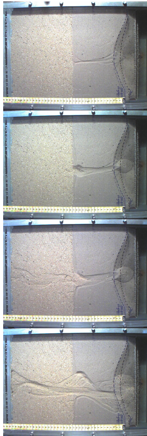
Fig 4 Channel formation in Masonry sand and Playground sand.
