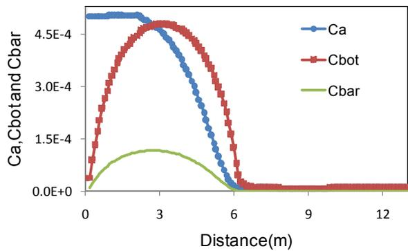
**Fig.7** Calculated profiles of concentrations with horizontal distance, in case with sediment diameter  $600 \mu\text{m}$ . Point  $x=6\text{m}$  is levee toe.
