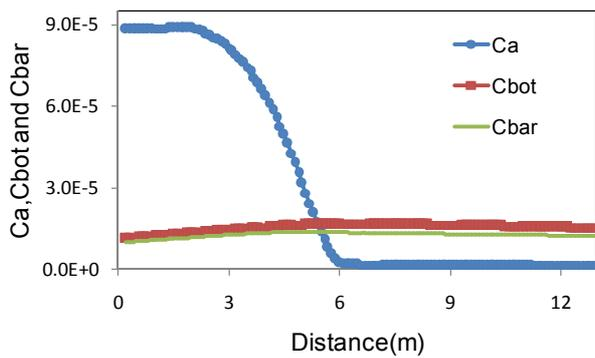
**Fig.6** Calculated profiles of concentrations with horizontal distance, in case with sediment diameter  $60 \mu\text{m}$ . Point  $x=6\text{m}$  is levee toe.
