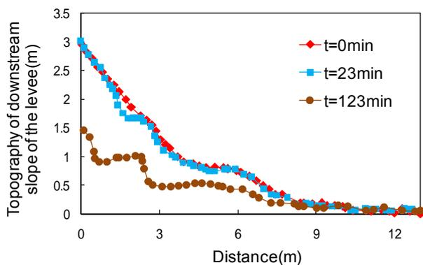
**Fig.2** Evolution of levee topography in the course of overflow experimentation after materials given by MLIT<sup>5)</sup>.
