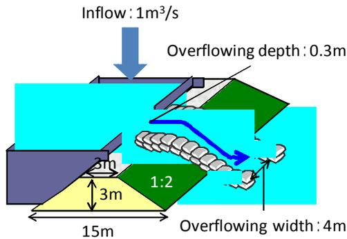
**Fig.1** Experimental setup of the levee scouring by overflow after materials given by MLIT<sup>5)</sup>.
