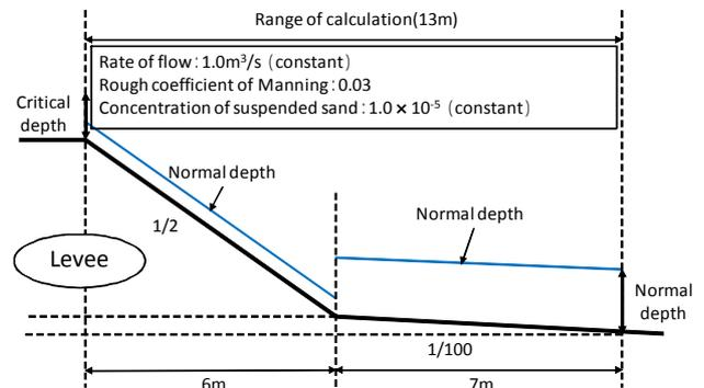
**Fig.5** Condition of calculation<sup>5)</sup>.
