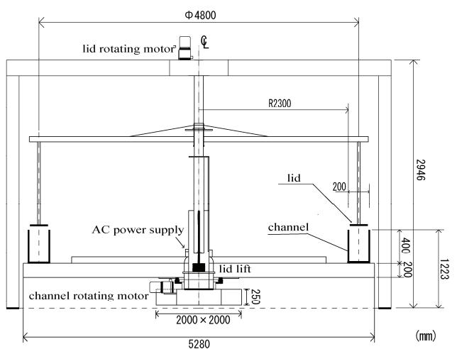
**Fig. 2** Cross section view of the annular flume
