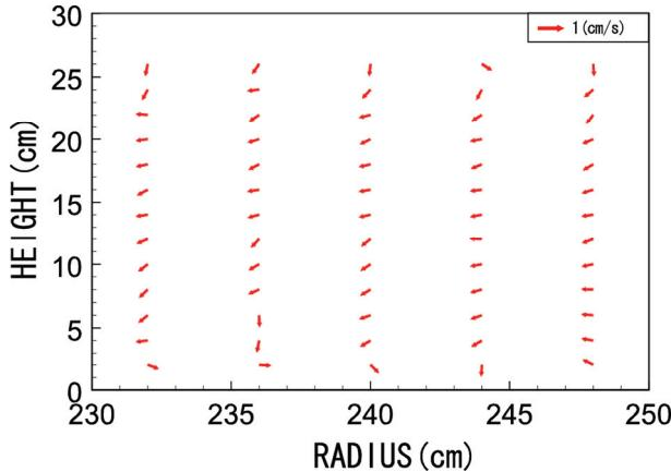
**Fig.5** The secondary flow field in the flume
