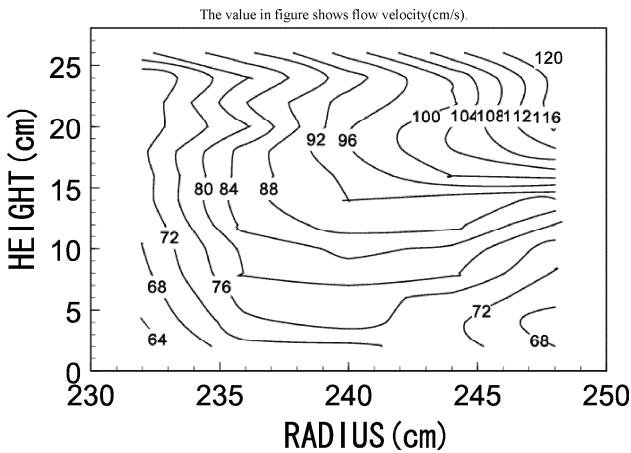
**Fig.4** The tangential velocity profile in the flume
