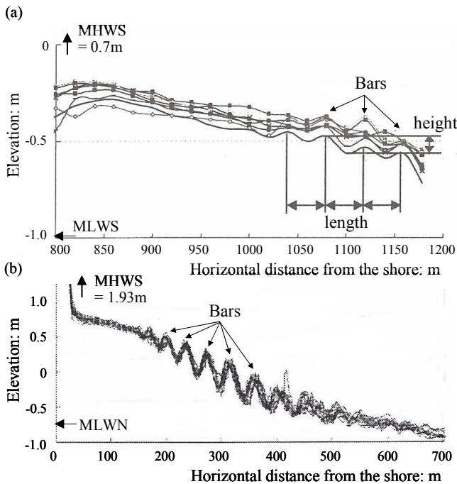
**Fig. 2** Results of field surveys showing the morphodynamic stability of intertidal sand bars at (a) Banzu sandy flat<sup>5)</sup> and (b) Okoshiki beach<sup>7)</sup>.
