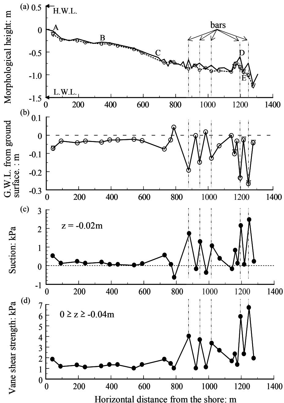
**Fig. 3** Results of field observations and surveys showing a close relationship between the variations in surface shear strengths and bar-trough morphology in the lower intertidal zone. The points marked A to E represent the locations of sediment sampling in Sassa and Watabe<sup>4)</sup>.
