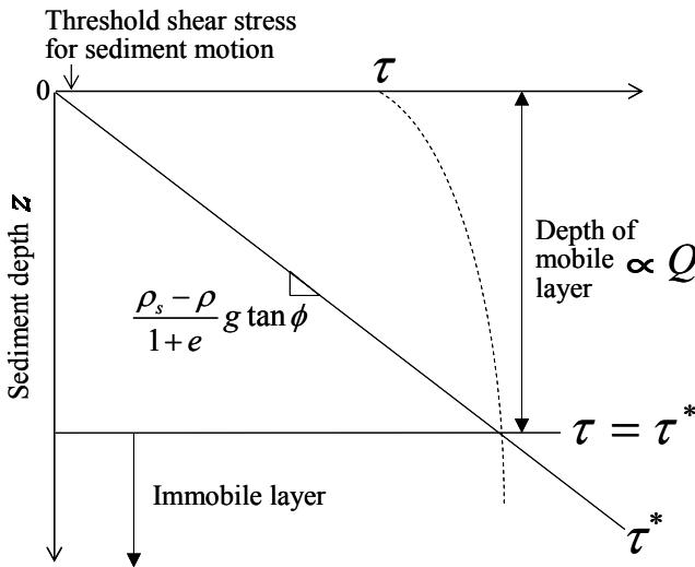
**Fig. 4** Sketch showing sediment transport rate  $Q$  as functions of both shear stress  $\tau$  and shear strength  $\tau^*$  of sediment. Here  $g$  is earth's gravity,  $\rho$  is mass density of fluid,  $\rho_s$  is mass density of sediment particles,  $e$  is void ratio of sediment and  $\phi$  is internal friction angle of sediment.
