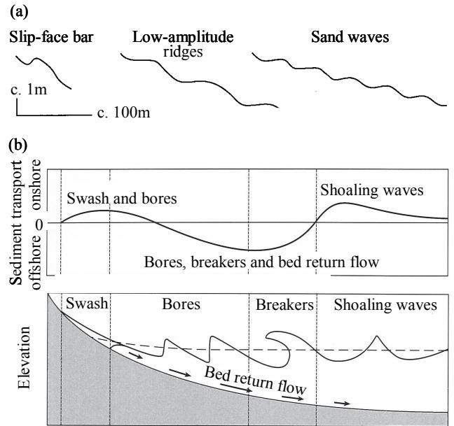
**Fig. 1** (a) Three main intertidal bar types; (b) sediment transport rate and direction associated with dominant hydrodynamic processes (adapted from Masselink et al.<sup>2)</sup>)
