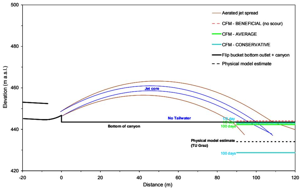
Fig. 6 Jet trajectory and scour formation in riverbed as a function of time duration of discharge (only CFM model): the LEFT hand side of the jet (largest trajectory distance). Comparison with physical model estimate of deepest scour in canyon.
