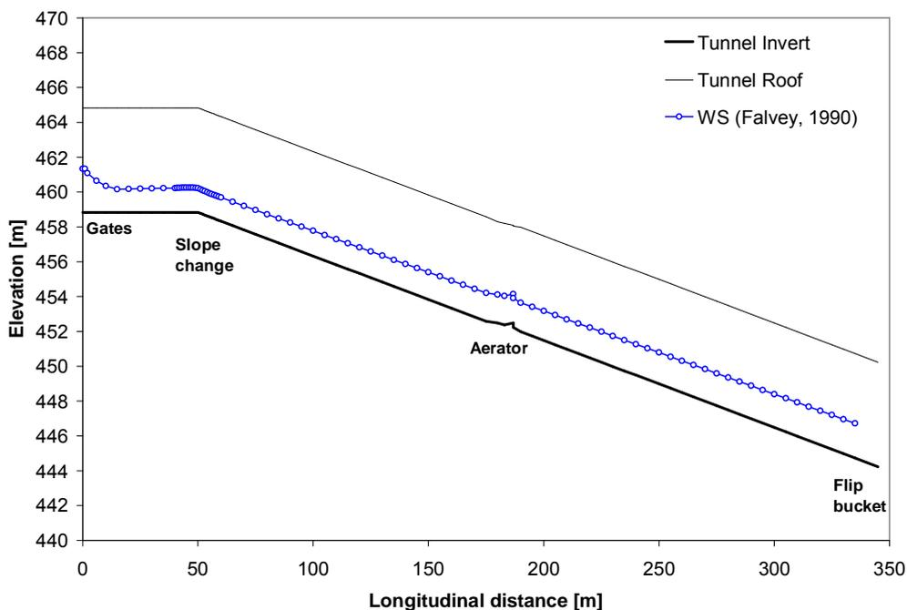
**Fig. 3** Water surface elevations along the bottom outlet tunnel (based on Falvey<sup>4)</sup>)
