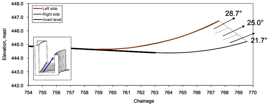
Fig. 5 Design of flip bucket: a) Plan view; b) Longitudinal profiles.
