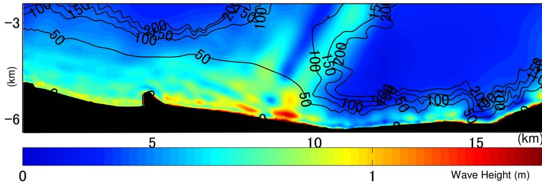
Fig.10 Predicted root-mean-square wave heights of long wave.
