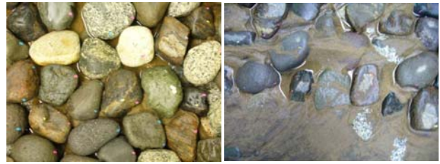
Fig.20 State of the river bed surface observed by hydraulic experiments designed to simulate a steep slope river with gravel or cobble as material-m.
