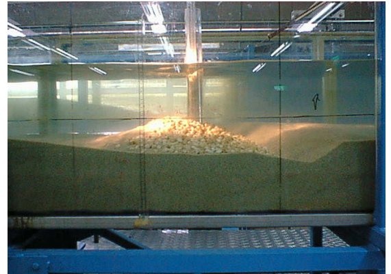
Figure 5. Formation of riprap mound around bridge pier in a degrading bed
