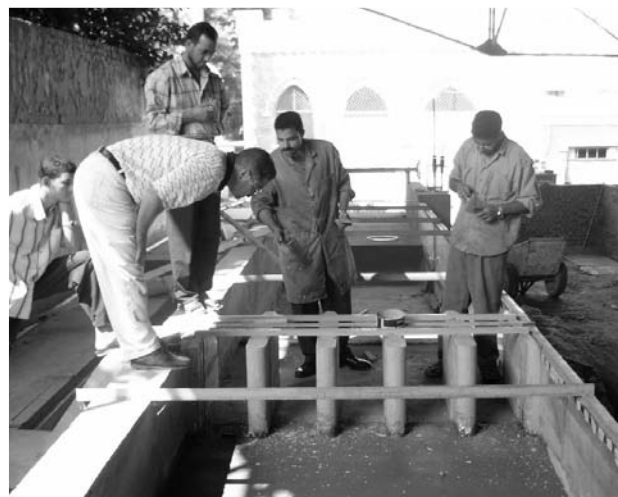
Figure 9 Scale model test for Rosetta Barrage: construction of the model at HRI
