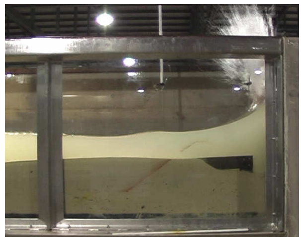
Figure 3. Wave breaking against a vertical wall. Metre stick gives scale
