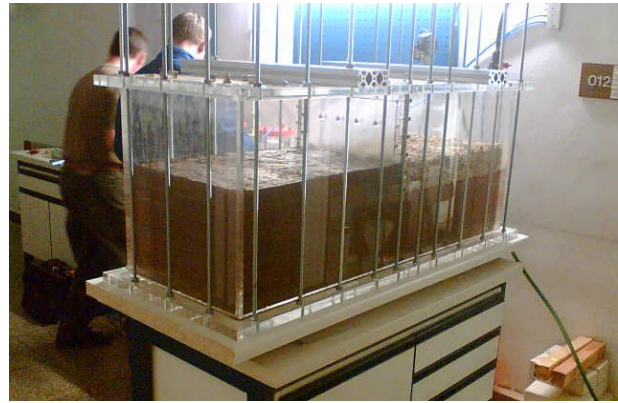
Figure 8. Experimental box with installed clay and filter material
