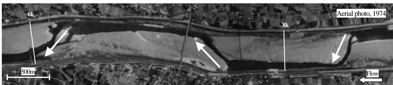
Photo 1. A typical example of crank flow (Down stream alluvial reaches of Naka river )
