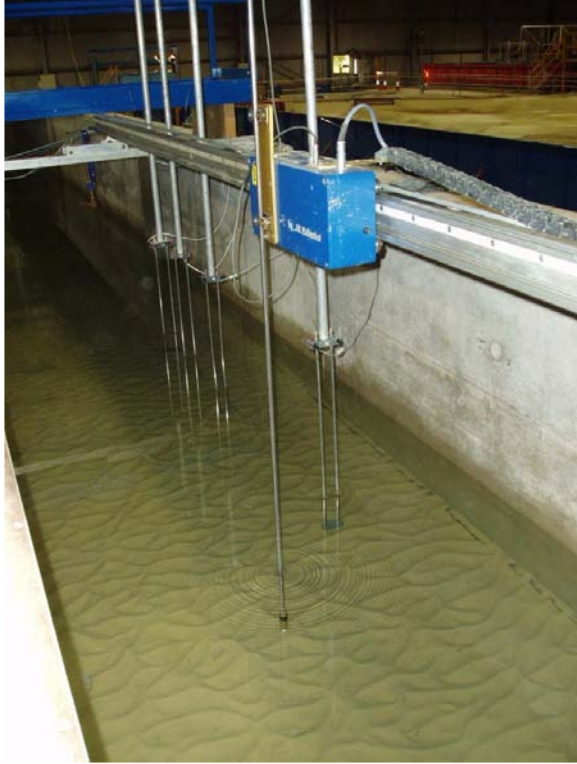
Figure 1. Bed profiler and wave gauges 5 to 8
