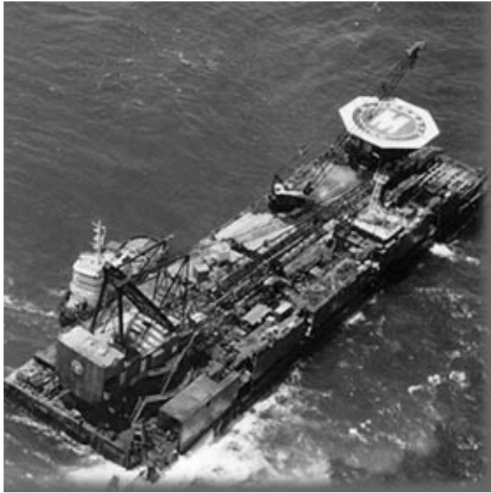
Fig 3. Pipelay barge LB 26 Pipes are welded along the starboard side of the barge
