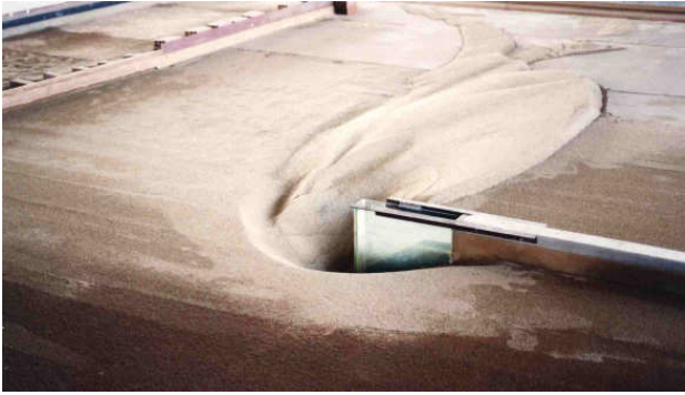
Figure 2. Scour hole in the reference test without protection [8].
