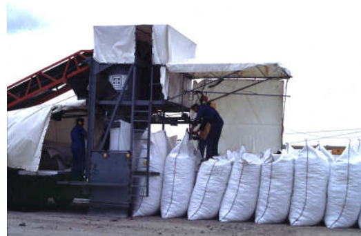
Figure 6. Filling plant for geosynthetic containers (1 m 3 )
