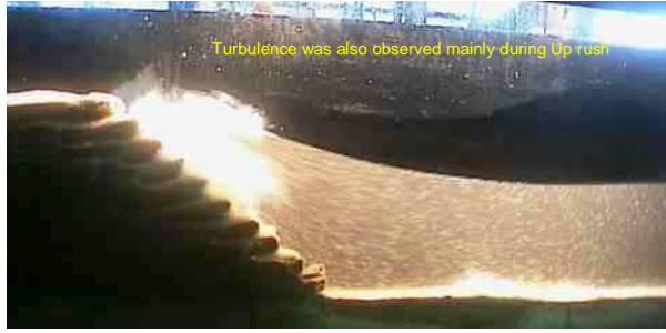
Figure 11: Turbulence During Wave Up and Down Rush of High Waves
