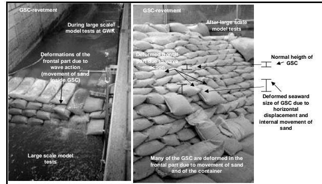
Figure 21: Displacement of Containers Observed During the Large-Scale Model Tests
