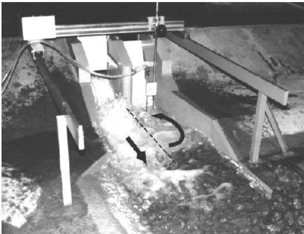
Figure 3. Original Design – Flow over a single spillway section, Q=312 \text{ m}^3/\text{s} , HTW = 437.7 m a.s.l. (regular tailwater level), gate opening a=4.0 \text{ m} ; the left margin of the main flow and a dominant vortex in an inactive half of the stilling basin can be clearly seen.
