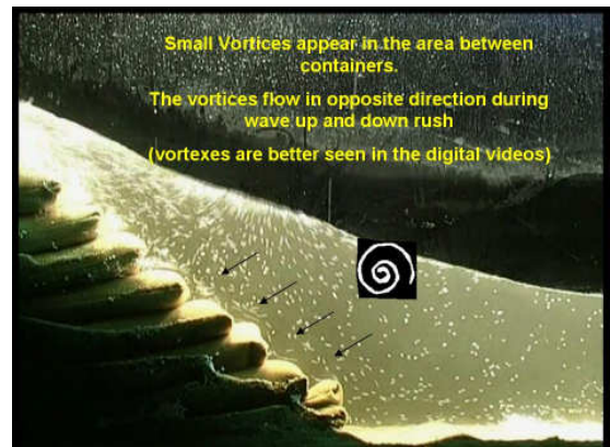
Figure 9: Vortices Appearance During Wave Up and Down Rush
