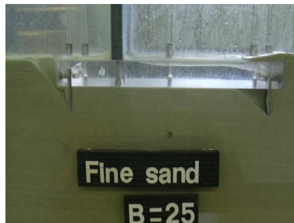
Figure 7. Observed phenomena during piping erosion: system without (top) and with cut-offs (bottom)
