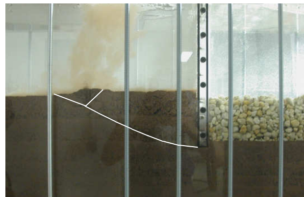
Figure 9. Result after failure (white line = slip plane)
