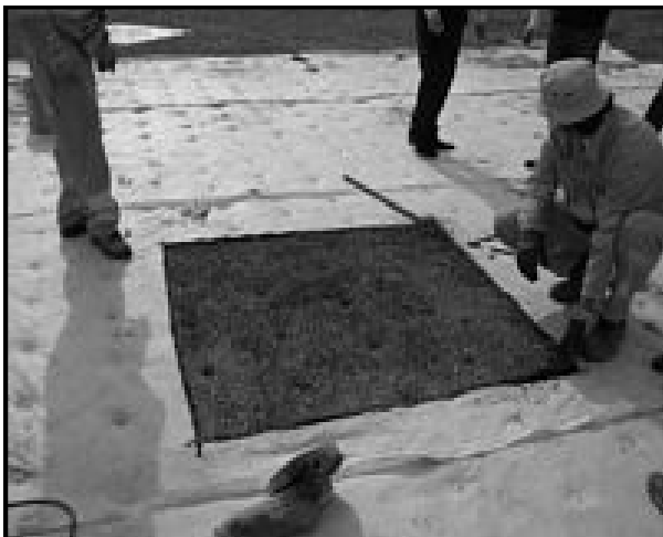
Figure 13. Extraction of samples for laboratory testing
